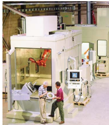
Among the advanced plasma control options available with Net Energy are the integrated PC/PLC-based Model 7700 UPC (above) and the unique Model 7700 PlazJet II, a high power plasma spray system.
